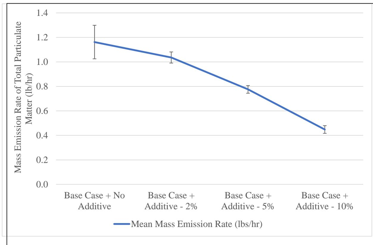
**Figure 8:** Abatement Effects of the Mineral Additive on the Mass Emission Rate of Total Particulate Matter (lb/hr) at Four Mix Levels (0%, 2%, 5% and 10%)
