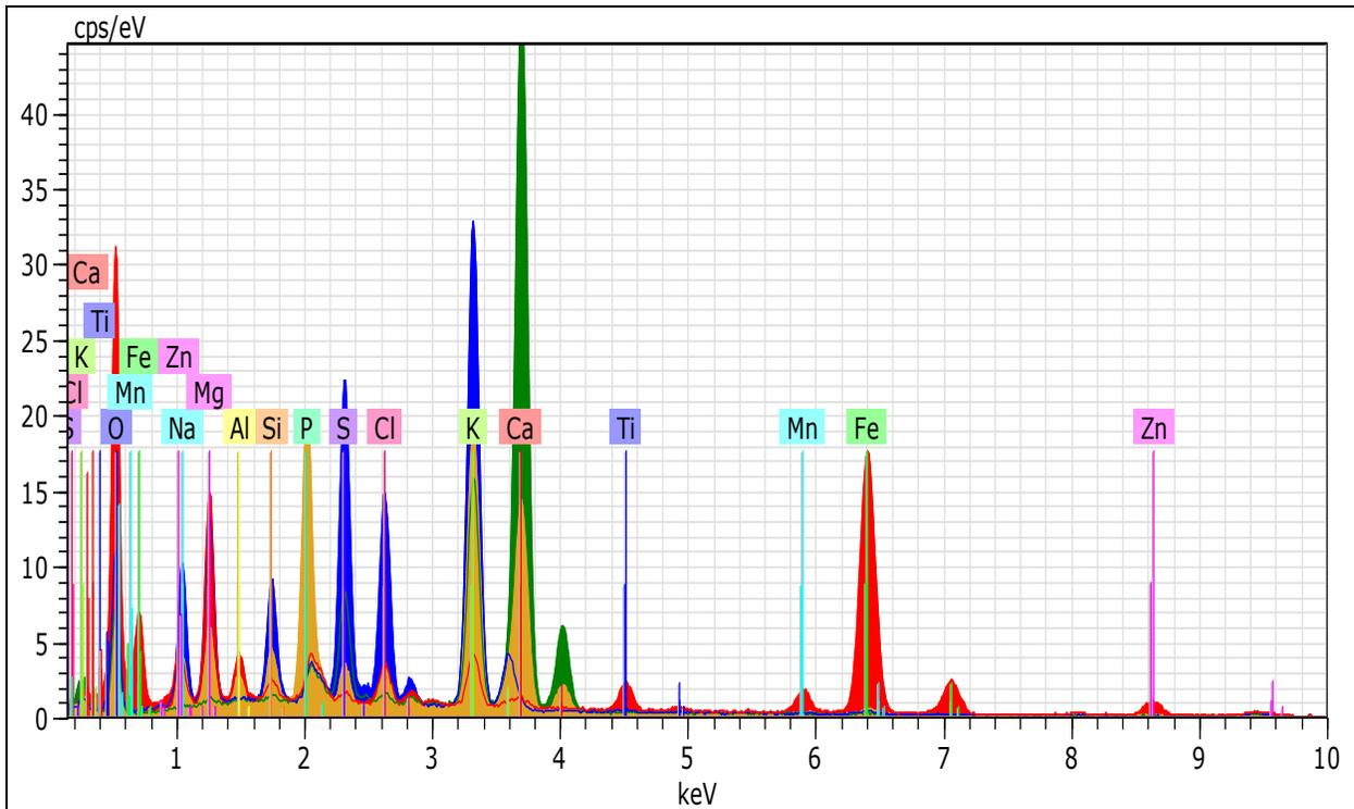
**Figure 12:** Graph of EDS Spectra of Bottom Ash from L1
