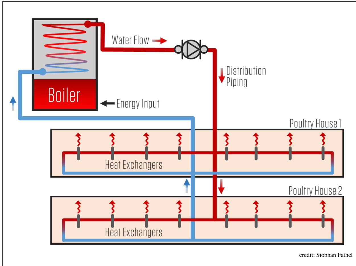
**Figure 2:** Representation of the Hydronic Heating Circuit at Site L1
