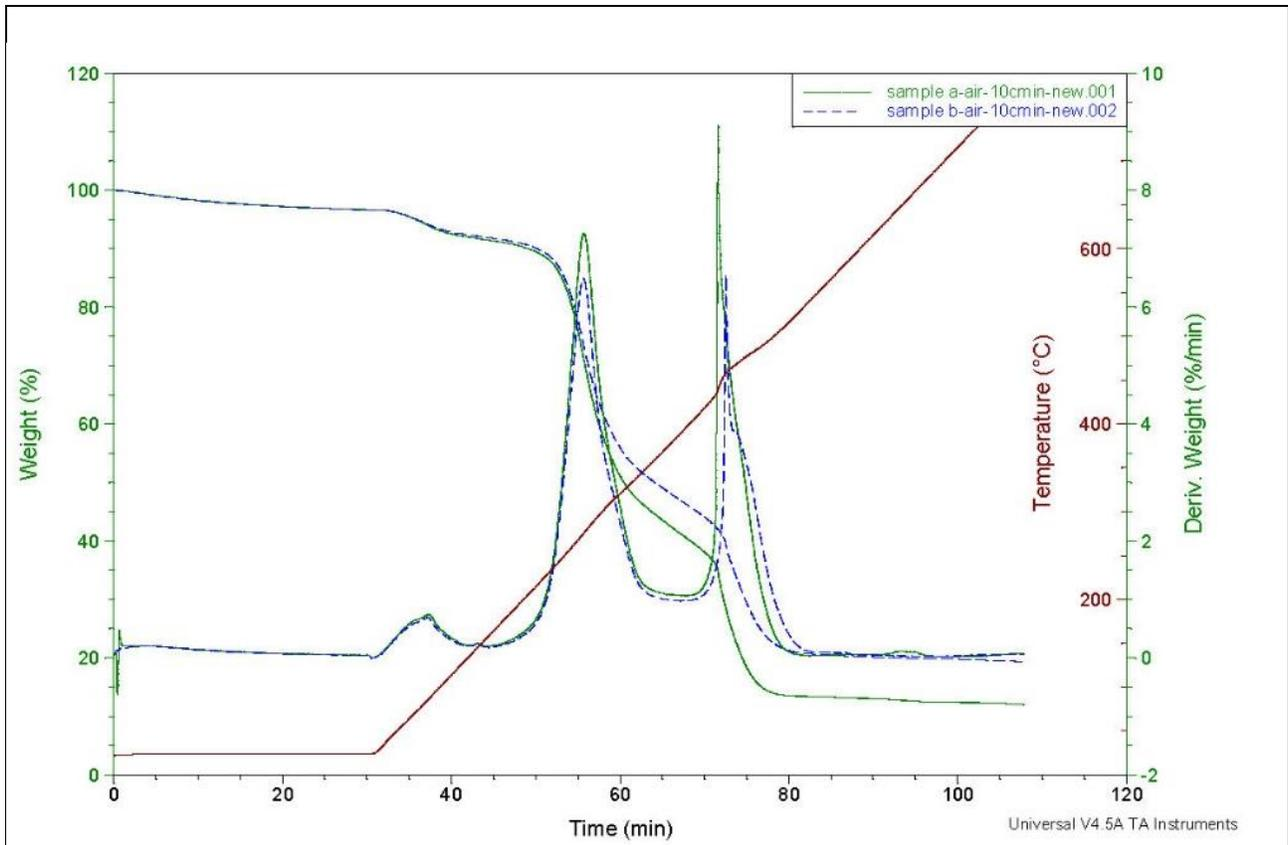
**Figure 6:** Overlay of TGA Curves for Samples A and B Versus Time Under Air Flow
