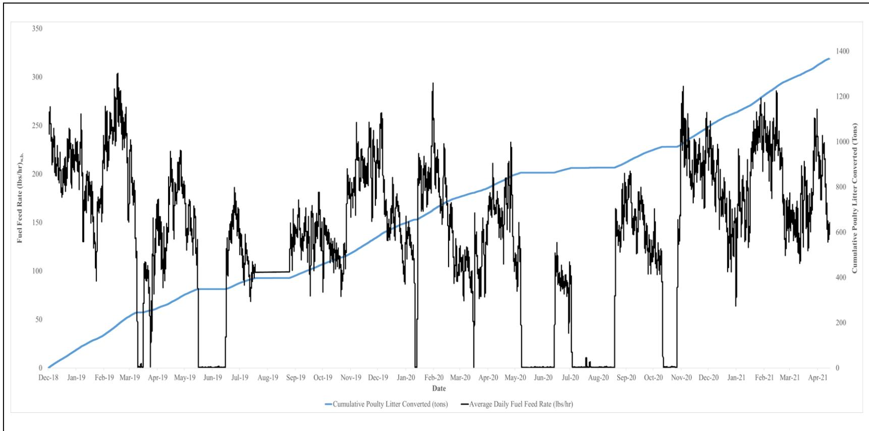
**Figure 7:** Average Daily Fuel Feed Rate & Cumulative Tons of Poultry Litter Converted from December 17, 2018 through April 30, 2021 at the L1 Site as Monitored by System Load Cell Dataloggers
