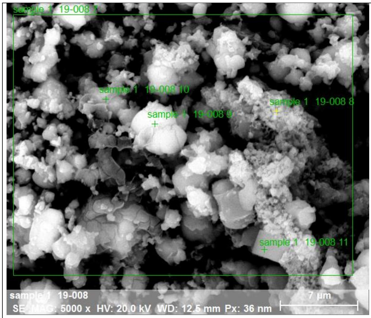
**Figure 9:** Filterable Particulate Matter at 5000x Magnification from Run 030119 – 4 from L1
