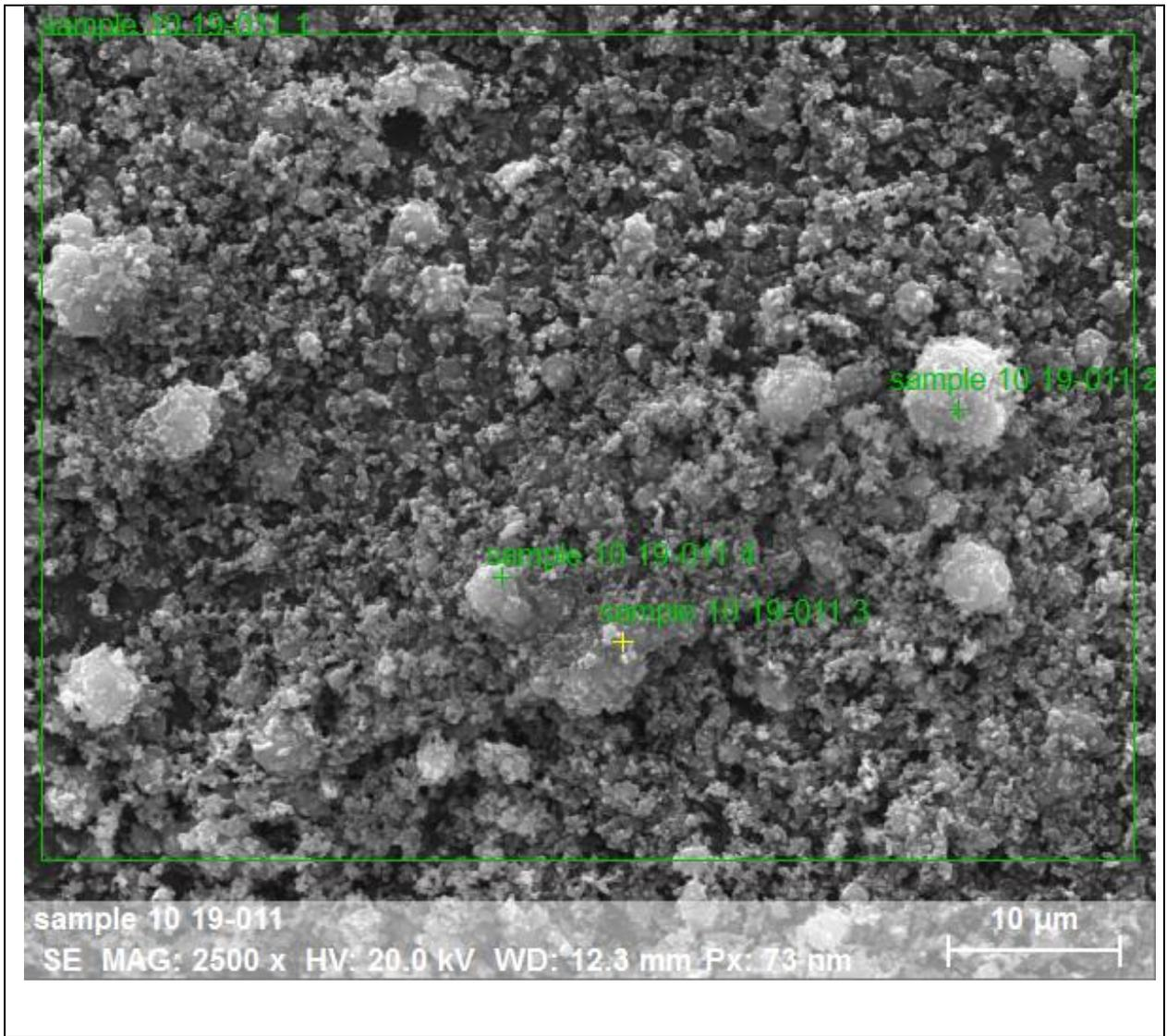
**Figure 15:** Filterable Particulate Matter at 2500x Magnification from Run 030519 – 2 from L2
