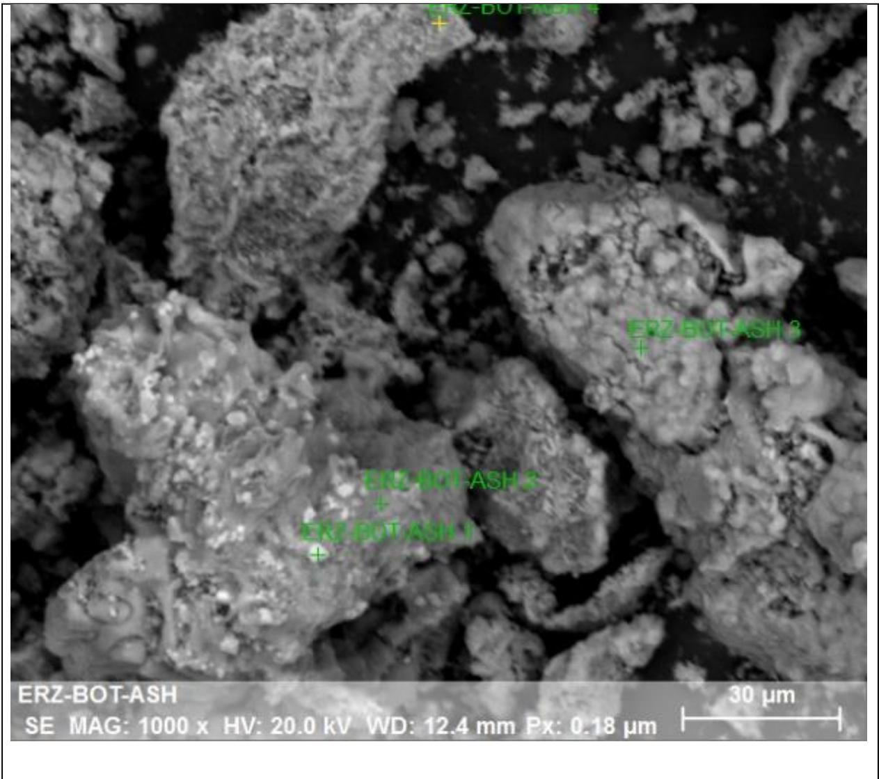
**Figure 11:** Bottom Ash at 1000x Magnification from L1
