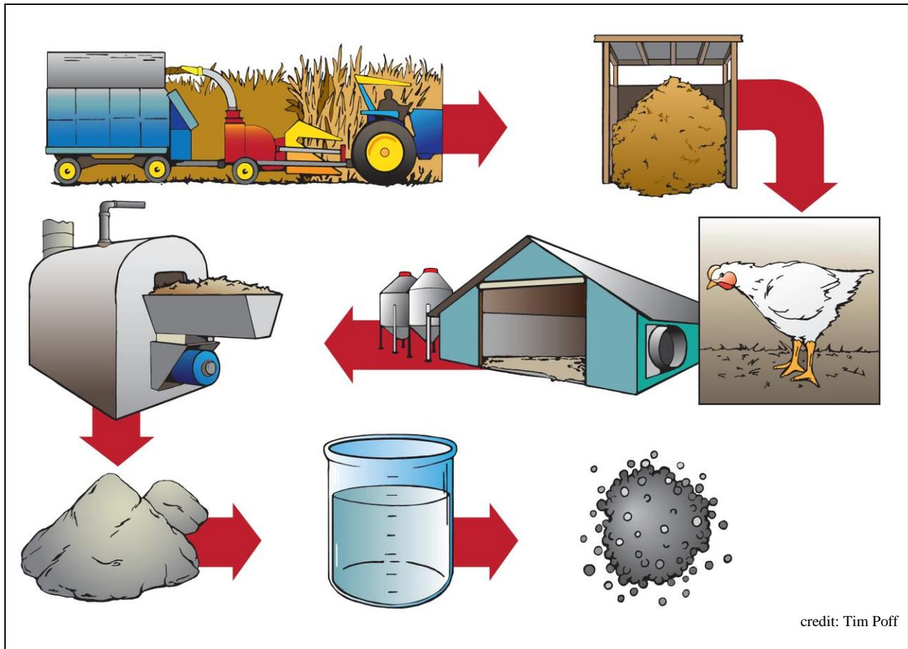
**Figure 4:** On-farm Biomass Feedstock-to-Bedding-to-Boiler-to-Byproduct System at L1 Showing Co-product Ash Processing for Value-added Product Development
