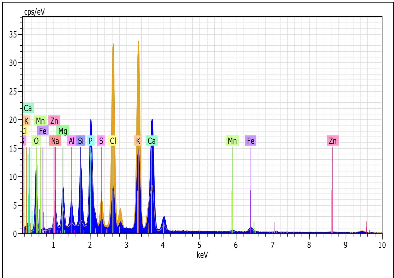
**Figure 14:** Graph of EDS Spectra of Fly Ash from Abatement Device from L1
