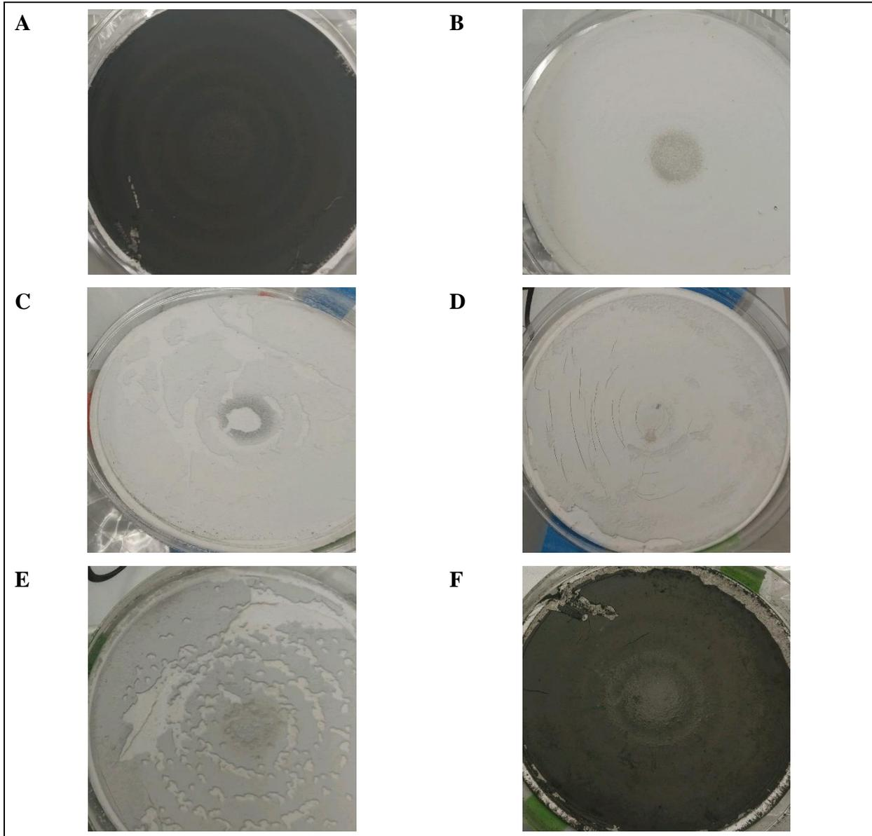
**Figure 17:** Pictures of Filter Media with Filterable Particulate Matter Catch for Wood with Cyclone (A), and Poultry Litter-Fired Runs with Cyclone Only (B), Wet Scrubber (C), and with Mineral Additive at 2% (D), 5% (E), and 10% (F)
