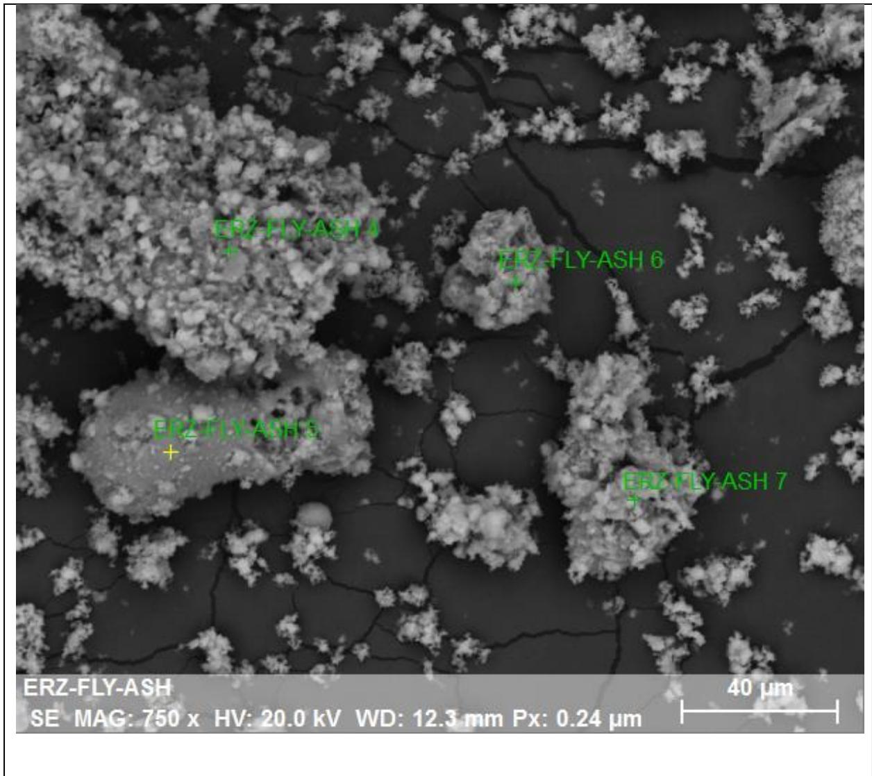
**Figure 13:** Fly Ash from Abatement Device at 750x Magnification from L1
