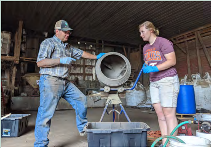
Mr. Earl Ray Zimmerman and Clara Ervin making granulated fertilizer from poultry litter ash
