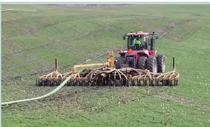
Agri-Applicators, Inc. are injecting 15,000-20,000 acres per year in South Central Pennsylvania with a drag hose system
