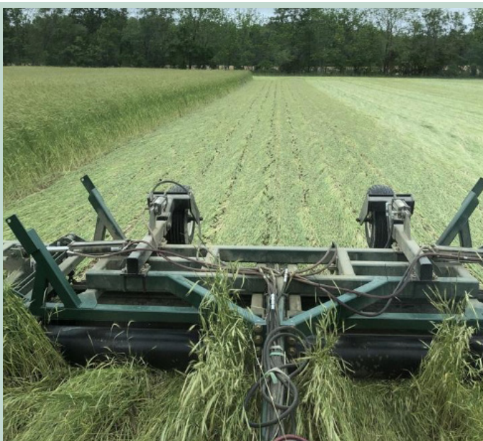
Figure 4 b. Roller/crimper used to terminate 6 ft tall, high biomass rye prior to planting.
