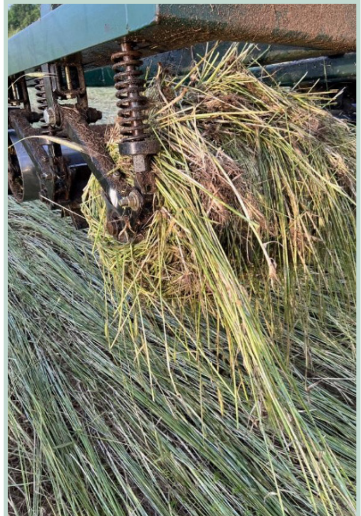
Figure 2. Crimping against the grain and on angled ends causes severe wrapping that required extensive downtime to address.
