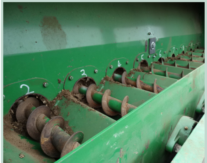
Photo above: The 14 ft. augers required excessive hydraulic power to function effectively. The augers have been cut down to about 30 in. at the front of the bed of the injector to maintain their metering and grinding functionality, while a drag chain was installed to do the majority of the litter movement with minimum energy (photo below).
