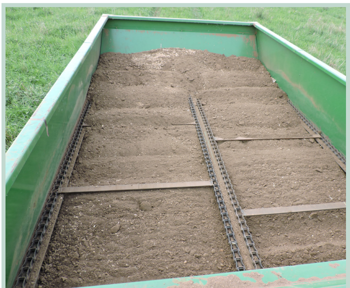
Photo above: Drag chains move litter from the back of the Subsurfer to the augers in the front.
