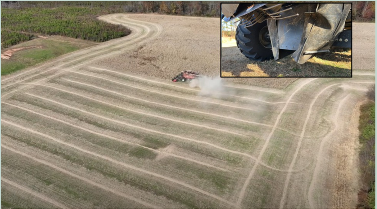
Figure 3. Chaff lines created during soybean harvest at Shepherd Grain Farms. Photo: Claudio Rubione, GROW. The inset photo features the chaff line distribution system mounted on the back of the combine.
