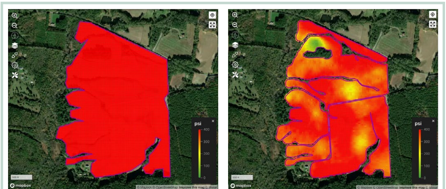
Figure 9. Soil compaction at 6 inches in FR1 in 2023 (left) and 2025 (right).
