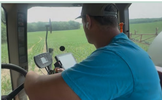
Figure 2: Once established, tramlines make it easy to see where to place equipment wheels, concentrating compaction due to heavy equipment in the tramlines, reducing soil compaction over the rest of the field.
